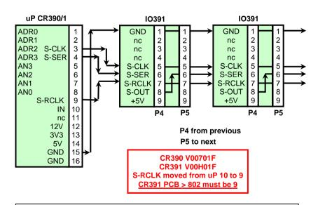
uP Control: Up to 6 Relay PCB daisy chained to uP
