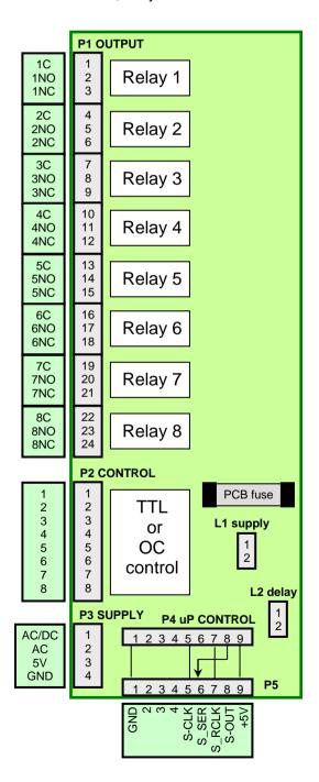
L1 selects TTL supply from on-board regulator, via AC supply (P3-3 and P4-9 not connected). L1 not installed, TTL supply from P3-3 or P4-9.
